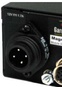
Fig 3.4b Dual-Source DC power input
